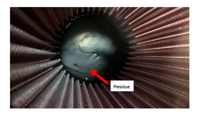
If loose residue is detected, remove it carefully prior to installation of the air filter.
